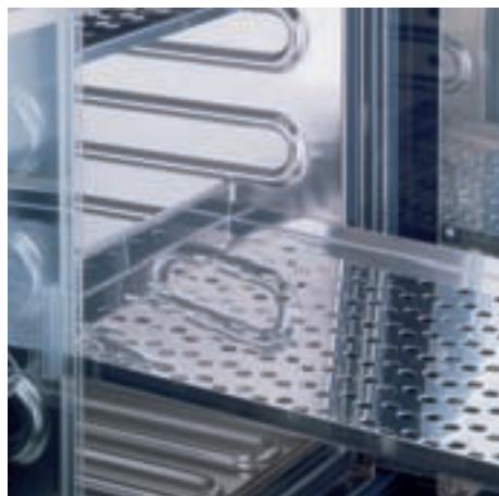
A Memmert special: the all-round heating is located below deep-drawn ribs which carry the non-tipping stainless steel shelves and at the same time ensure optimal and particularly gentle heat transfer to the incubator load.
