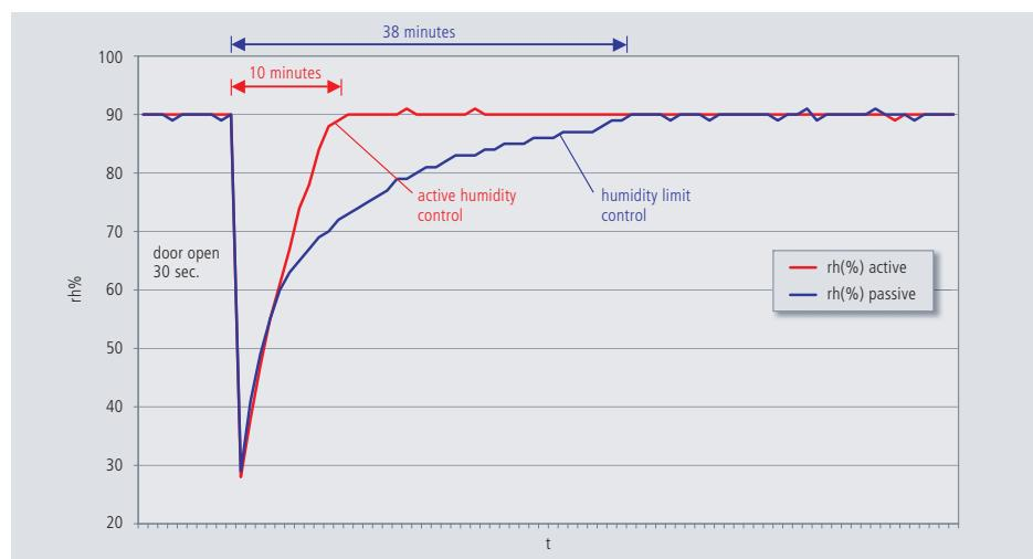
The difference in humidity recovery time between humidity limit control and active humidity control (example: INCO/108).
