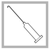
2. Insert a clean delivery tube into the lodate-lodide Titration Cartridge. Attach the cartridge to the Digital Titrator.
