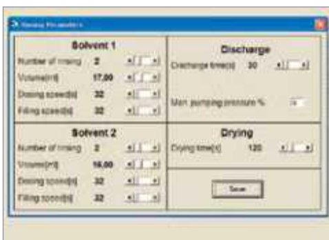
Each rinse/dry step can be individually pre-selected. Even the application dependent quantity of solvent and the drying time can be separately determined.
