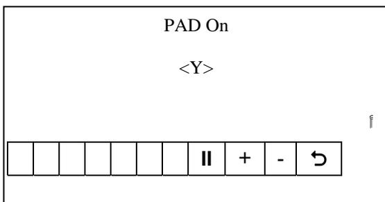
The auxiliary pump (“PAD” pump for demineralised water) is to be activated if the pressure of the demineralised water is less than 1 bar.
