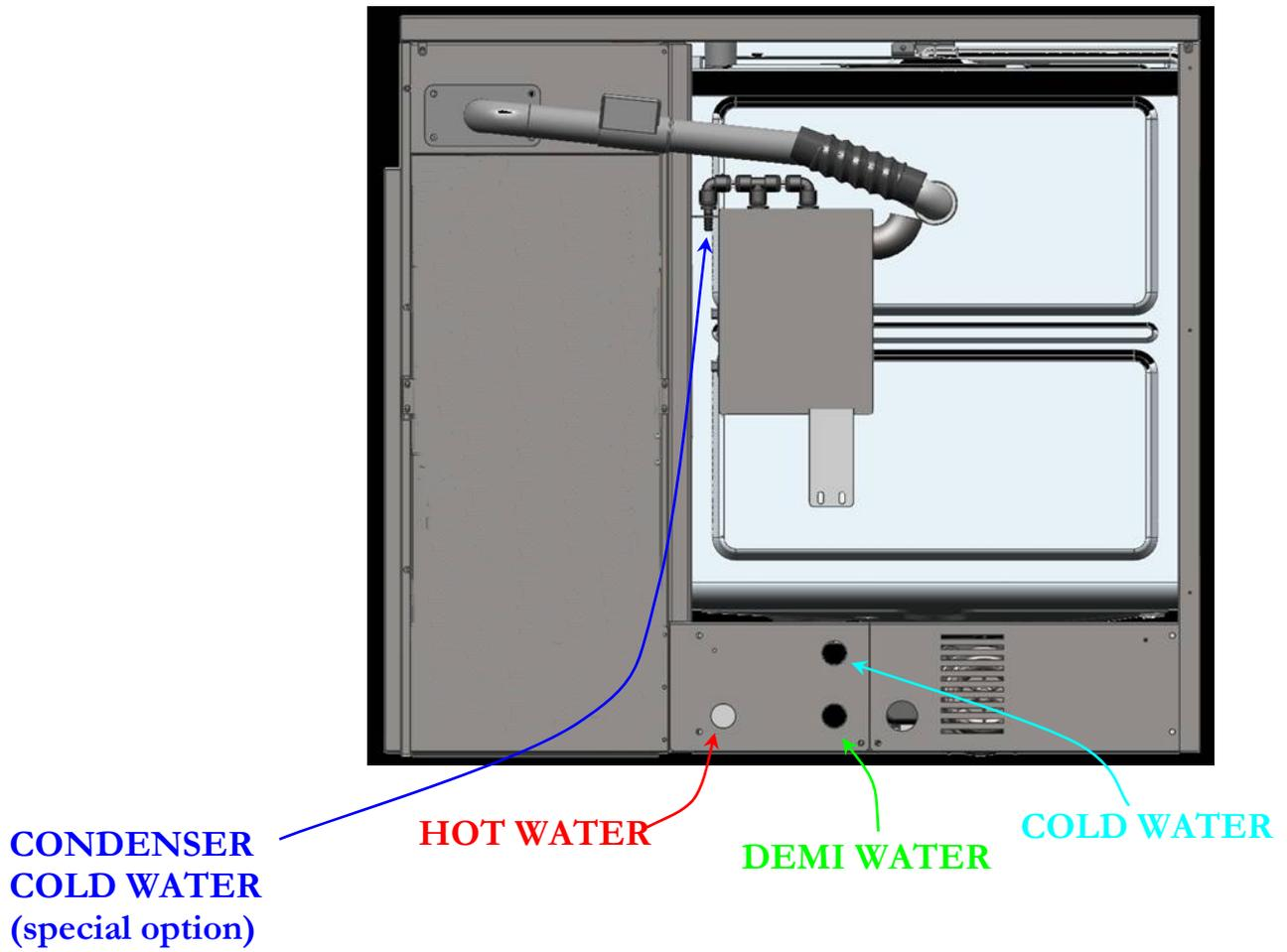
If the connections are made to new pipes, it is advisable to allow the water to flow through in order to eliminate any rusty deposits or sludge.
