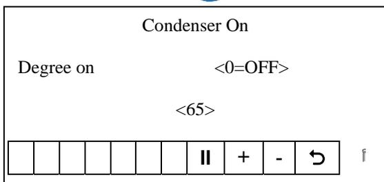
The steam condenser can be inhibited by entering a temperature of 0°C.If a temperature is entered, that will be the temperature at which the condenser starts operating.
