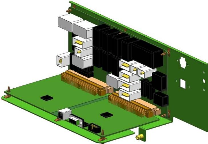
The rack has two electronic boards joined by connectors: motherboard and daughterboard.
