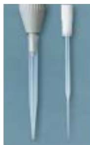
Use of a glass Pasteur pipette with the adaptor supplied, even when protection filter installed.
