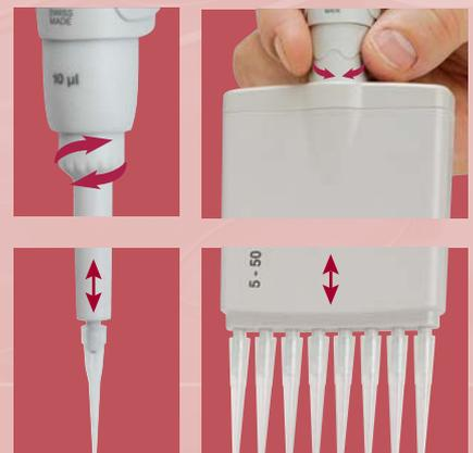
Bowed shape of ejector head adds to effortless, easy sequential tip ejection on multichannel models.
