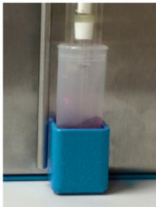
3. Place the clip (C) over the back of the stand so that the end of the electrode enters the storage tube and is fully immersed in the storage solution. You may need to adjust the liquid level or the clip height for optimum depth.
