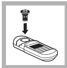
3. Insert the TNT/COD Adapter into the cell holder by rotating the adapter until it drops into place. Then push down to fully insert it.
