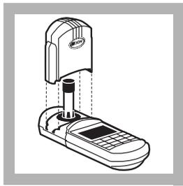
**13.** Place the control vial in the cell holder. Tightly cover the vial with the instrument cap.
