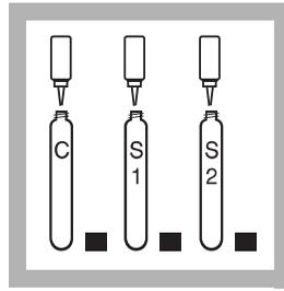
**11.** Add 2 drops of Accelerator Solution to each vial. Cap and invert to mix.
