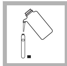
4. Fill a Test 'N Tube vial with deionized water. Label this vial as the "blank". Wipe the outside of all the vials with a tissue to remove fingerprints and smudges.
