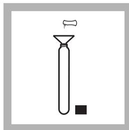
7. Label a vial "control." Open one ToxTrak Reagent Powder Pillow and add the contents to the empty reaction vial.
