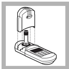
5. Place the blank in the adapter. Tightly cover the vial with the instrument cap.
