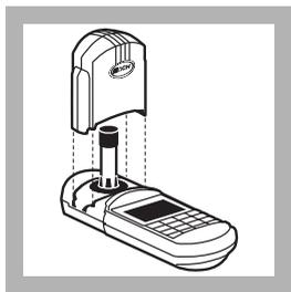
**17.** After the absorbance of the “control” vial has decreased  $0.60 \pm 0.10$  absorbance units, place the blank in the adapter. Tightly cover the vial with the instrument cap.
