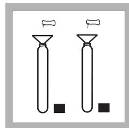
8. Label each sample or dilution vial clearly. Add the contents of one ToxTrak Reagent Powder Pillow to each labeled vial.
