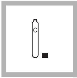
**9.** Add 5.0 mL of deionized water to the control tube.
