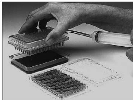
6. Now, slowly lift the Vaccu-Pette/96™ from its resting position on the 96 well plate, at the same time depressing the syringe plunger to zero. By the time the plunger is at zero, the Vaccu-Pette/96™ tips should be clear of liquid in the 96 wells.
