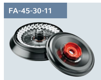
30 x 1.5/2 mL micro tube rotor with aerosol-tight lid for safe centrifugation of hazardous samples. Max. speed 20,800 x g (14,000 rpm).
