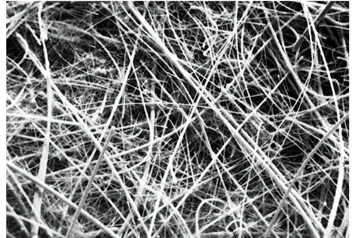
Glass microfiber filters are manufactured from 100% borosilicate glass.
